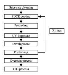
Figure 2. The manufacturing process of color filters
