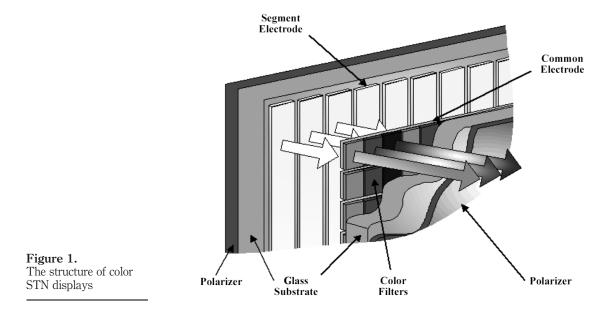
displays, each pixel is divided into R, G and B sub-pixels. Controlling the light through the color filter allows different colors to be produced through combinations of the primary colors. Figure 2 illustrates the manufacturing process for color filters.
